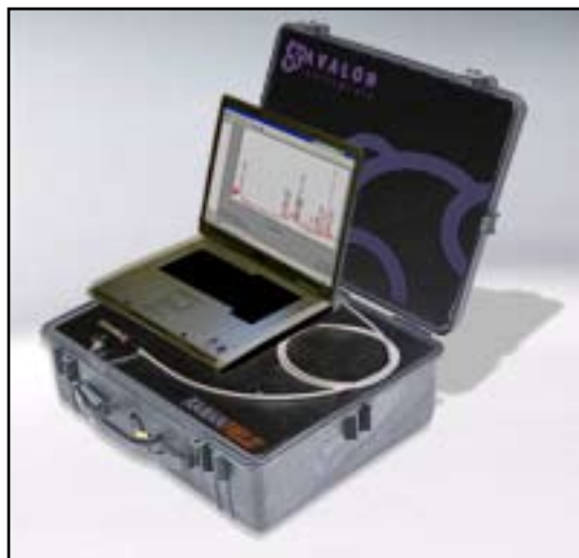
Figure 5a Portable RamanField suitable for on-site.
