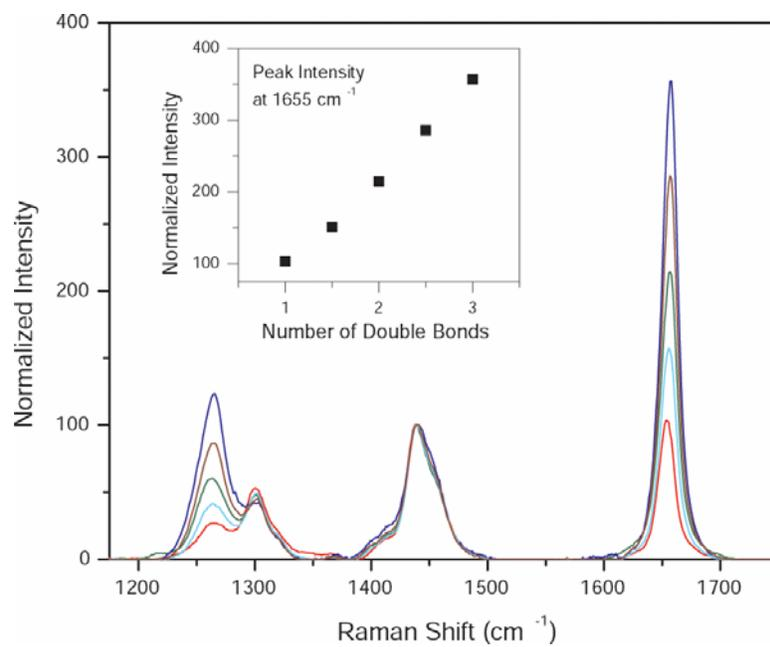
**Figure 1.** Raman spectra of oleic (red), linoleic (green), linolenic (blue) acids and 1:1 mixtures of oleic:linoleic (cyan) and linoleic:linolenic (maroon). Inset: Quantification of double bond content at 1655 cm<sup>-1</sup>.
